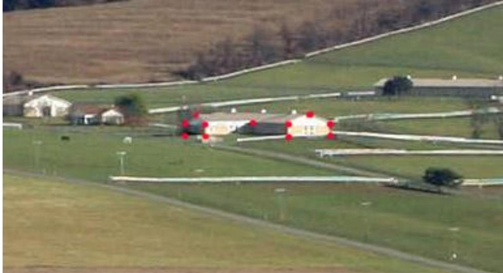
While it is not optimal to use match-points near the terrain (due to the fact that finished floor elevation in a CAD model may differ from where the structure actually hits the terrain) because both the structure type and distance from the camera, there are very few options for good match-points.
